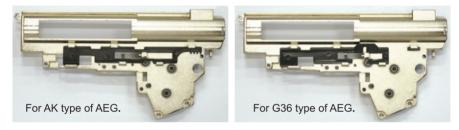
**4.** Remove the cut-off lever, and replace it with the polymer cut-off lever provided with your ASCU-V3. Replace the cut-off lever spring. Use the original screw.
