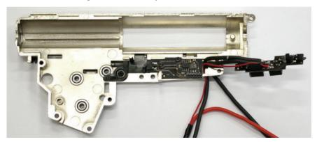
7. Place over & connect the ASCU Mosfet to the ECU. Be carefull to connect accurately the connecting pins of the ECU and Mosfet Boards.
