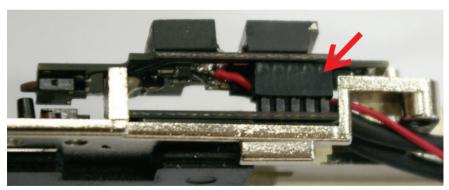
8. When connecting the two boards connect the pins EXACTLY as it is shown on the picture above.
