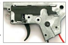
As there are slight differences in the triggers between the different manufacturers, if your trigger is not engaging the trigger switch properly, then you can use the provided trigger extension:
